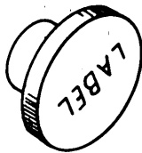
Figure 6-11. Example of Label Placement Which Can Result in Upside-Down Position (Ref. 4)
