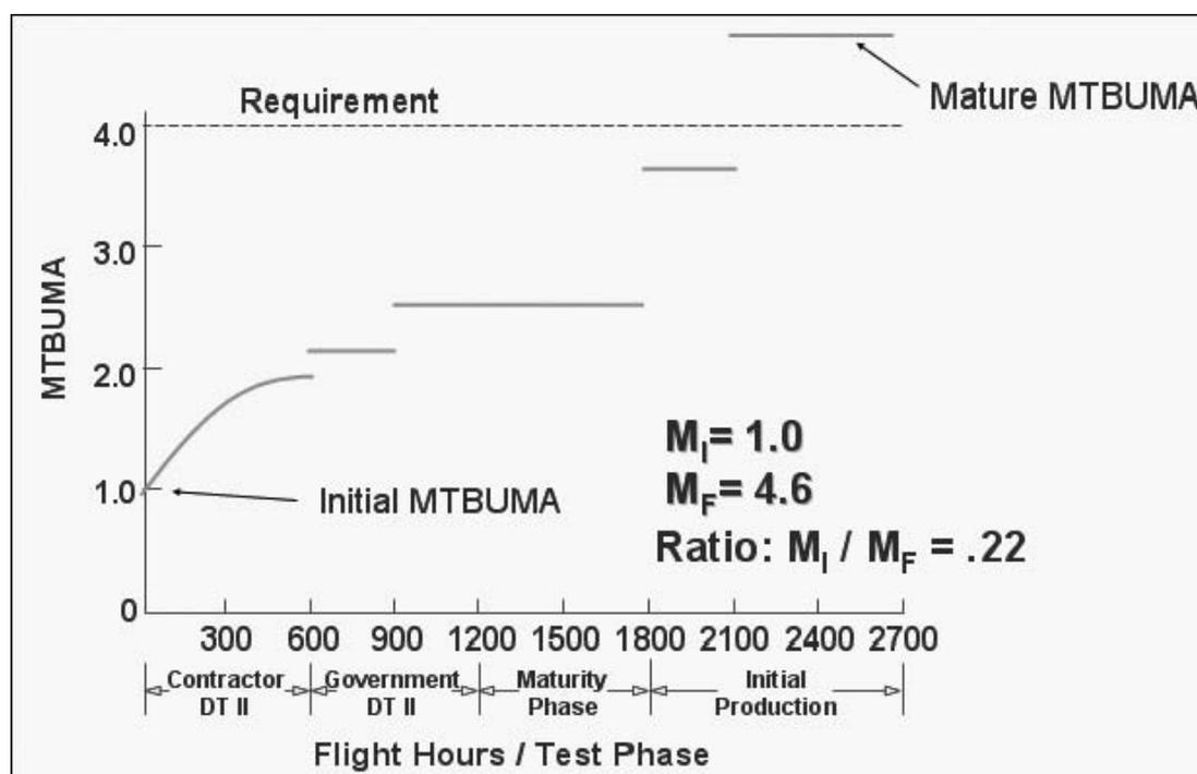
Figure 1. The Blackhawk helicopter reliability growth measured in meantime between unscheduled maintenance action (MTBUMA) per flight hours per test phase
