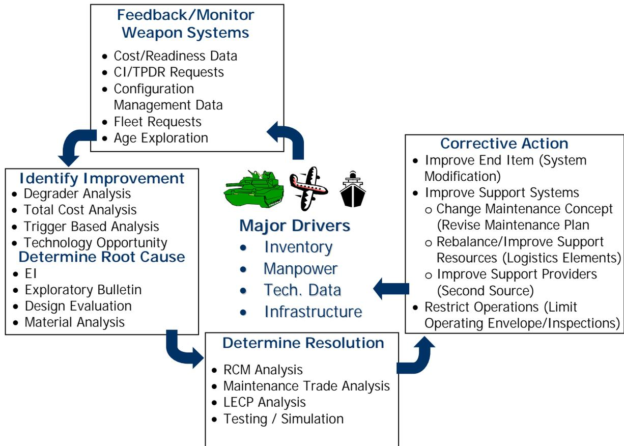
**FIGURE 3.7. RCM Sustained Maintenance Planning in Modification Environment**
