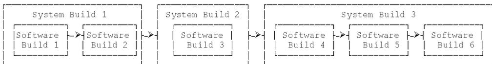
FIGURE 1. Example showing how system and software build strategies can differ.
