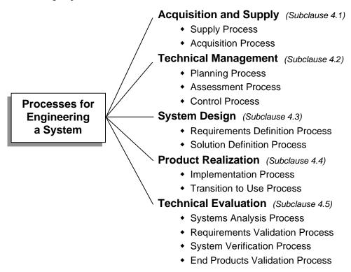
Figure 1.2—Fundamental processes for engineering a system
