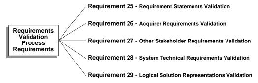
Figure 4.5.2—Requirements Validation Process requirements
