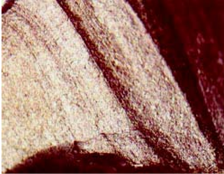
Figure 32 Characteristic Fatigue Striation Pattern 15
