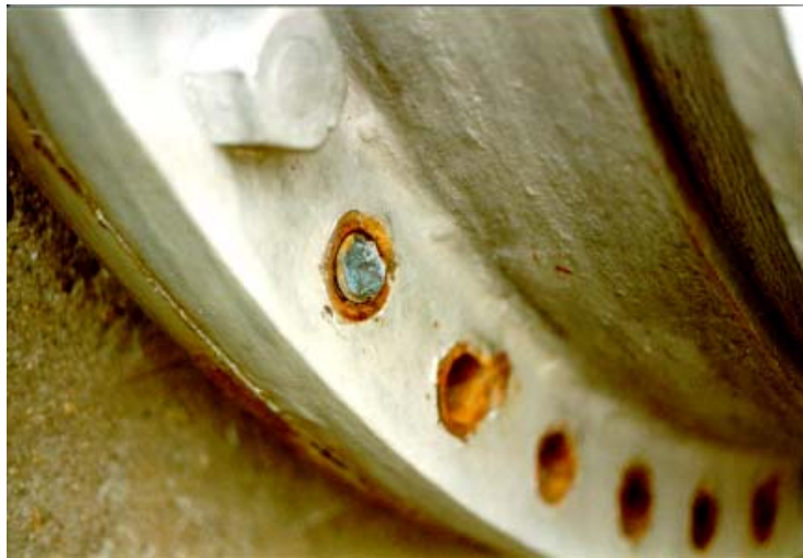
Figure 29 Dezincification of Brass Containing a High Zinc Content 13
