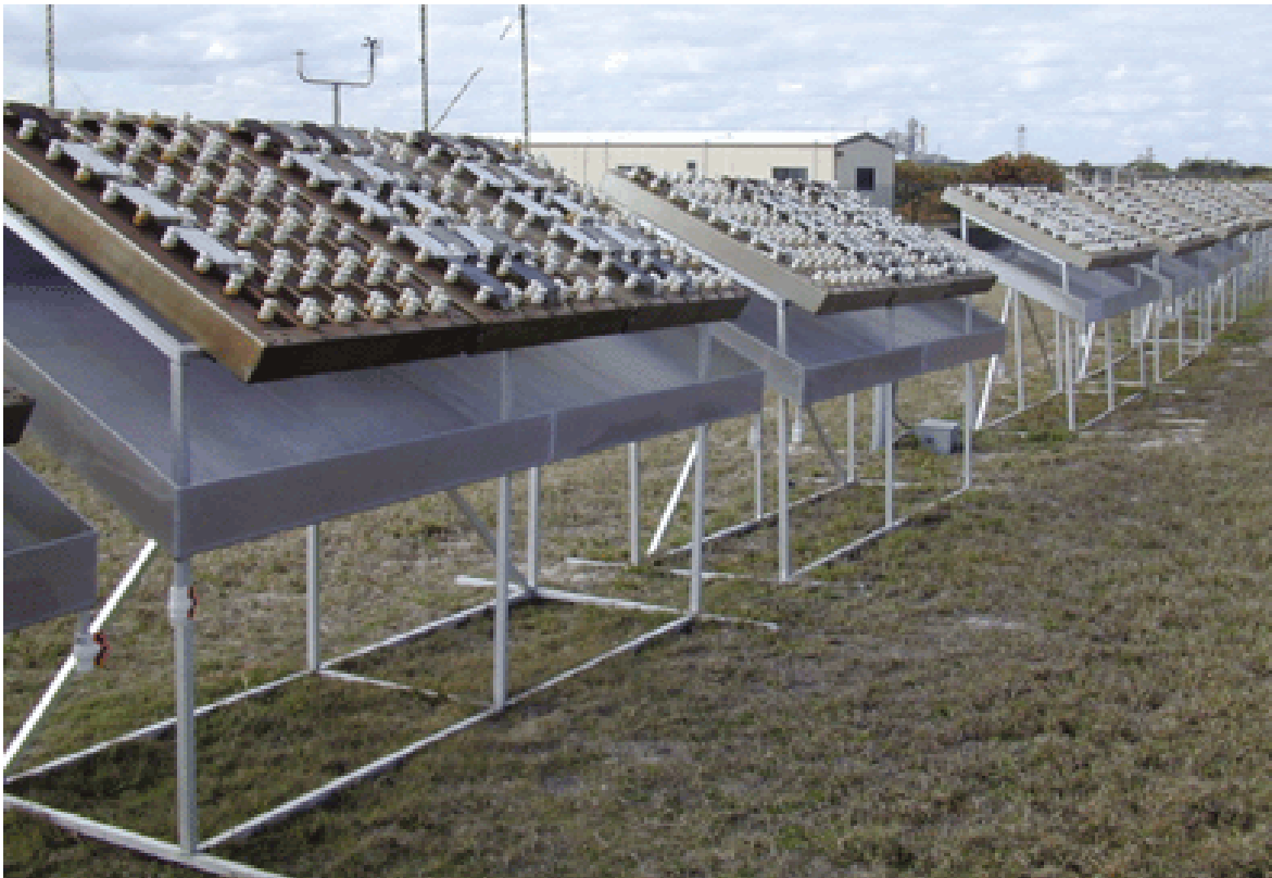
Figure 16 Atmospheric Corrosion Test Rack 2
