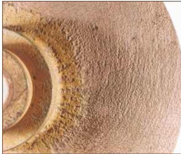
Figure 11 Erosion Corrosion of a Brass Pump Impeller
