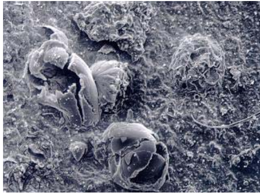
Figure 41 Tubercles as a Result of MIC (courtesy of Metallurgical Technologies, Inc.) 28
