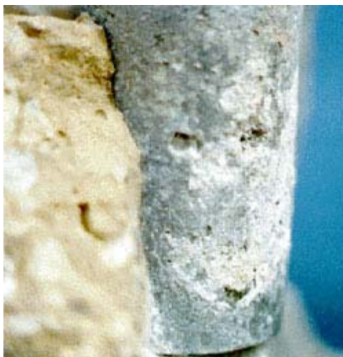
Figure 27 Pitting Corrosion of an Aluminum Railing near the Atlantic Ocean 2
