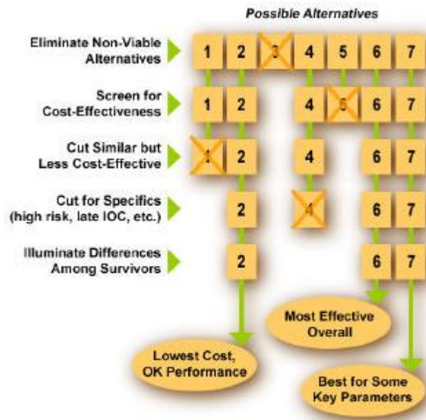
Figure 9-1. Eliminating Alternatives in an AoA
